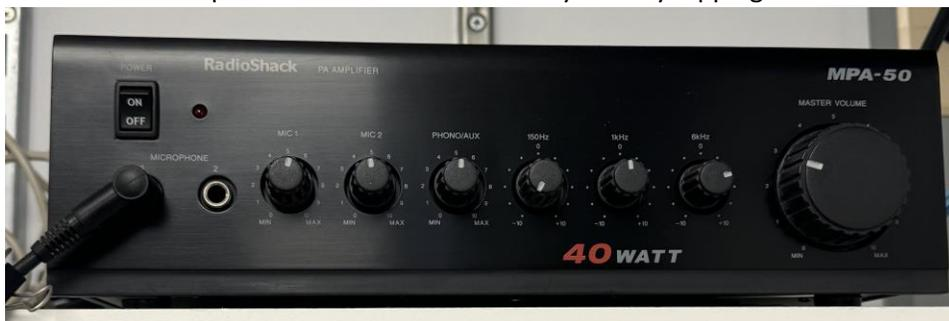
The red light will turn on indicating the audio system is powered on.
